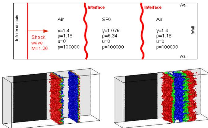
Figure 1: Geometry of the double-planar RM case and volume fraction visualisations at two different time instants using the ILES code (CNS3D) [4]. The dark region shows the initial position of the two planar interfaces.
