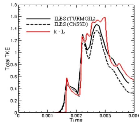
Figure 2: Evolution of the total turbulence kinetic energy in time: Comparisons of the  $k-L$  results with two ILES simulations using the CNS3D and TURMOIL methods.
