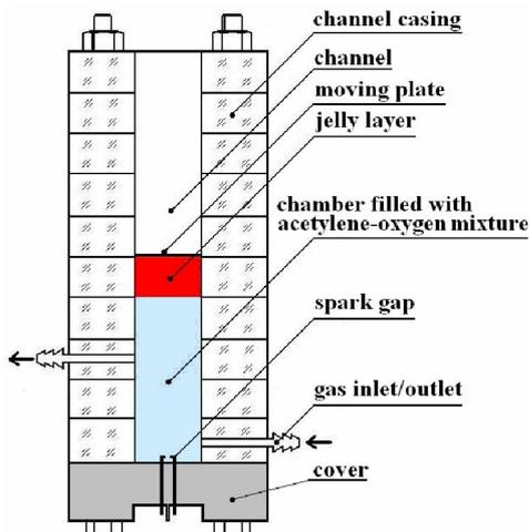
Fig.1. Schematic of experimental facility
