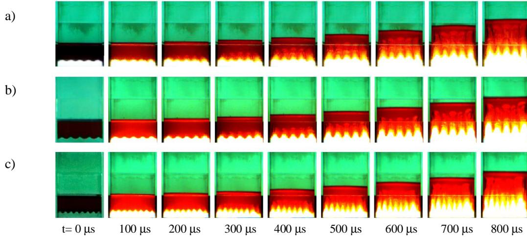
Fig.3. Photochronography of the jelly layer accelerated by the gas explosive mixture products.
