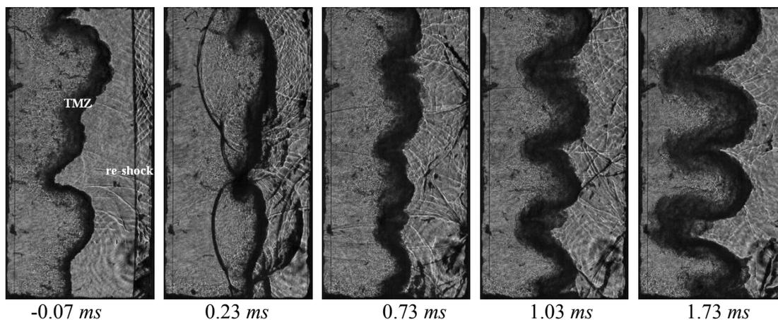
**Fig.4** Schlieren images of evolution of TMZ with two mode by re-shock
