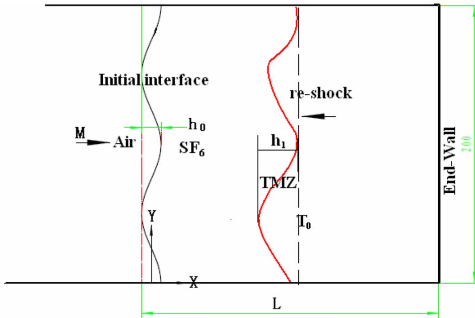
$M$  - the incidence shock Mach number;  $L$  - the length of the initial  $\text{SF}_6$  section;  $h_0$  - the initial perturbation width;  $h_1$  - the width of TMZ, when re-shock arrived at the TMZ;  $T_0$  - zero time when re-shock arrived at the TMZ.
