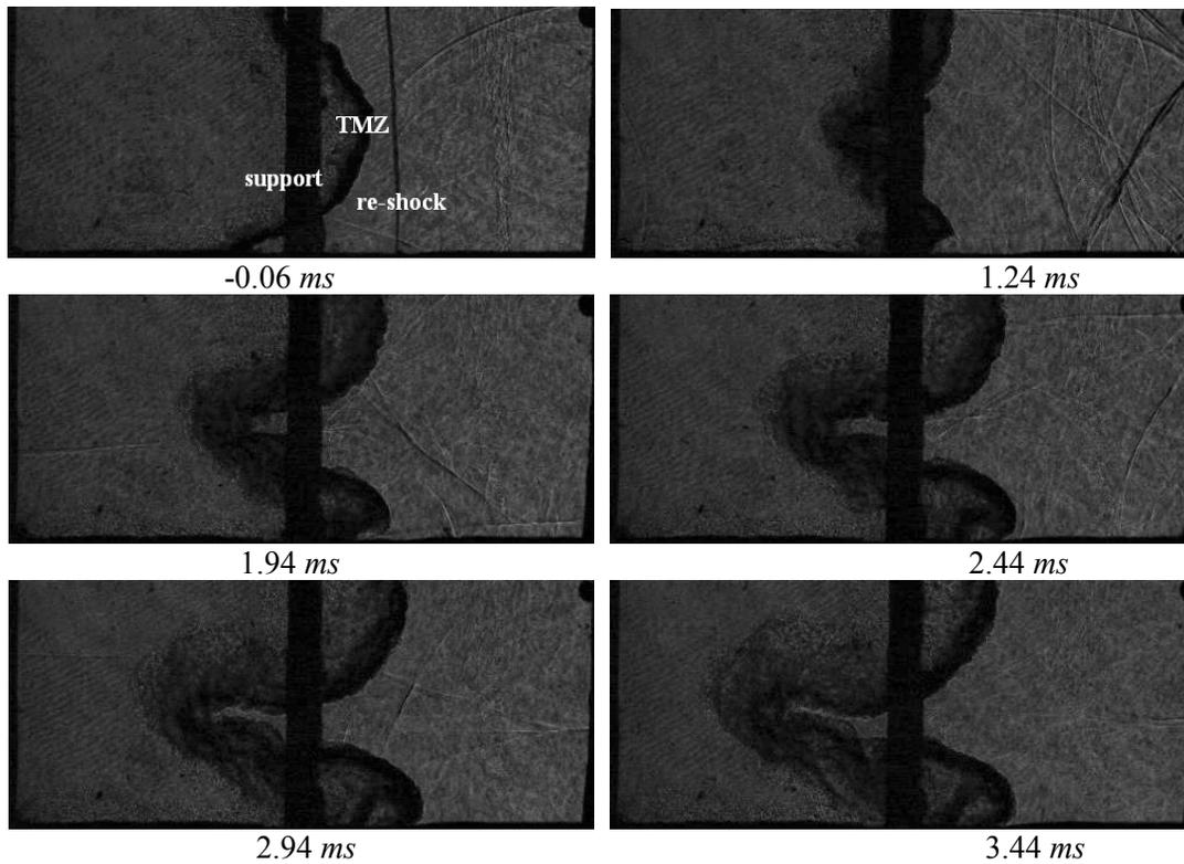
**Fig.2** Schlieren images of evolution of TMZ with single mode by re-shock
