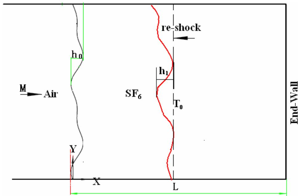
M - the incidence shock Mach number; L - the length of the initial SF<sub>6</sub> section; h<sub>0</sub> - the initial perturbation width; h<sub>1</sub> - the width of TMZ, when re-shock arrived at the TMZ; T<sub>0</sub> - zero time when re-shock arrived at the TMZ.
